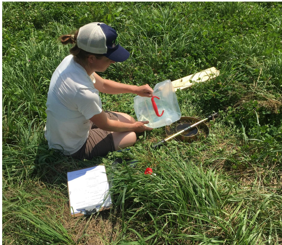
Using a double-infiltration ring to measure water infiltration rate in a field.
