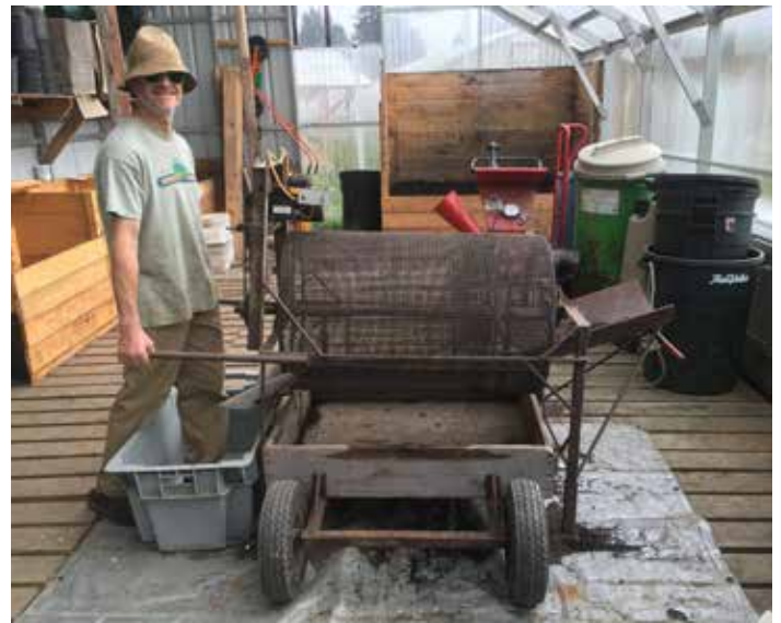
Above: Demonstrating the handles on the rear of the sifter that make it easy to transport
